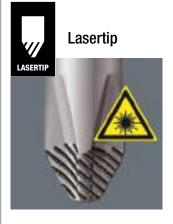
A precisely-focused laser creates a sharp-edged surface structure. This laser treatment results in an edge hardness of up to 1000 HV 0.3. Wera Lasertip "bites" itself into the screw head and prevents any slips out of the recess. It is available for screwdrivers for slotted, Phillips and Pozidriv screws.
