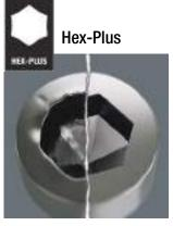
Hexagon socket screws are a problem, because the contact surfaces that transfer the force of the tool to the screw are very narrow. The consequence: the head of the screw can be damaged, usually rounding out the recess. Hex-Plus tools have larger contact surfaces to prevent this, driving from the
