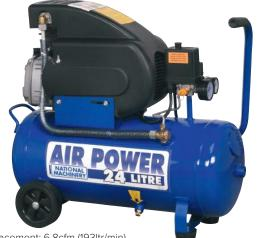
Air Displacement: 6.8cfm (193ltr/min). Maximum Free Air Delivery: 4.6cfm (130ltr/min). Maximum Pressure: 116psi (8bar). Aluminium cylinder head with cast iron
