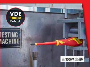
All of our insulated tools pass exhaustive testing to the international standard IEC 60 900 and the European standard for testing insulation to 1000V DIN 60 900.
