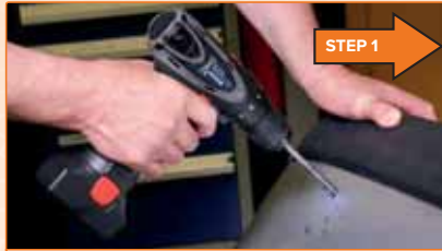
Drill 8mm pilot hole.
